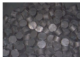
Briquettes made from sludge for recycling
