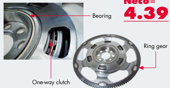
▲ One-way clutch and bearing imbedded in ring gear driven by the starter motor
