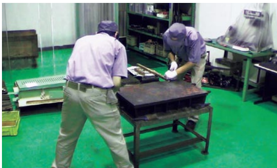
Photo 2: Practicing scraping by hand to create a very smooth surface that is not possible using a machine
