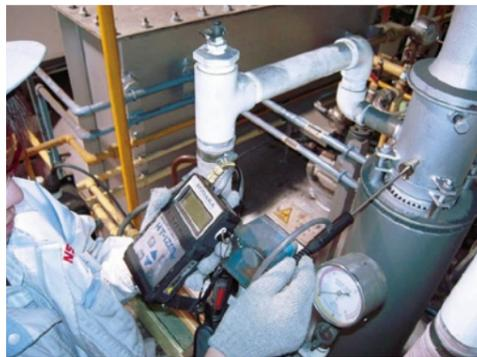
Measuring exhaust gas and optimizing firing conditions
