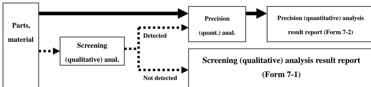
**Fig. 1 Analysis flow of substance testing applicable to ELV and RoHS**
